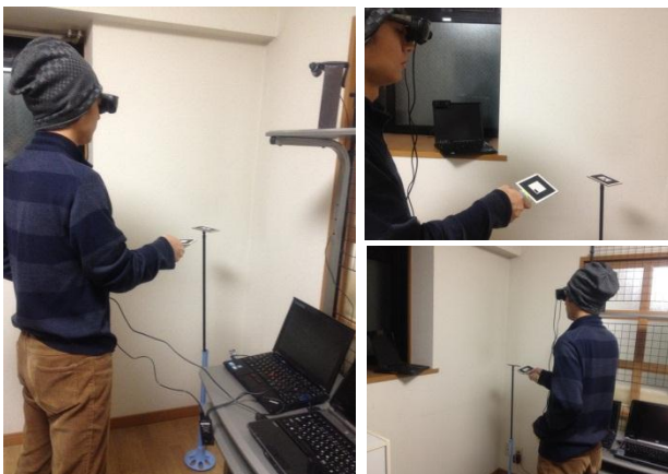
Figure 6. Operation scene. The user wore a HMD and grabbed the weapon marker in one's hand. Multiple cameras capture the video.
