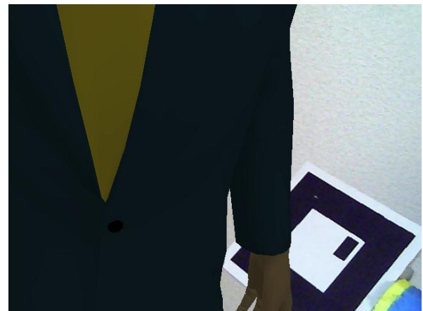
(a) Result without complement of marker information. Since the weapon marker went out of sight of HMD cameras, the virtual weapon could not be displayed.
