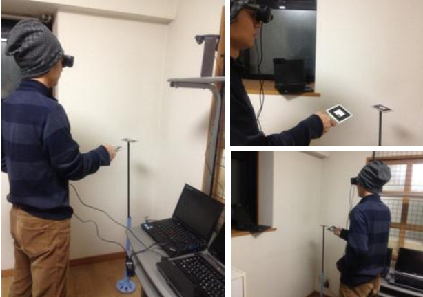
Figure 6. Operation scene. The user wore a HMD and grabbed the weapon marker in his hand. Three cameras capture the action.
