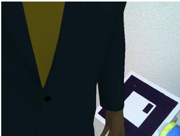
(a) Result without the complement of marker information. Since the weapon marker went out of sight of HMD cameras, the virtual weapon could not be displayed.
