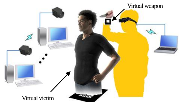
(b) After overlaid. A video captured with multiple cameras. The virtual victim and the virtual weapon are displayed on the positions of the markers in the video.
