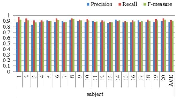
Figure 15: Performance of click gesture detection with the state transition model for the calculation task.
