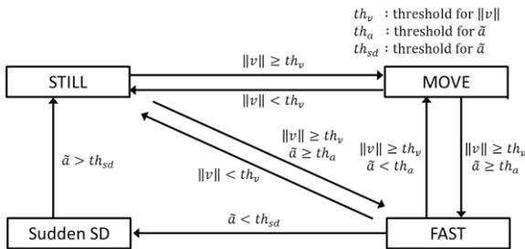
Figure 7: State transition diagram for detecting states of motion
