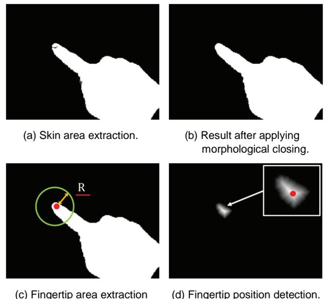
Figure 5: Hand area detection and fingertip position estimation.
