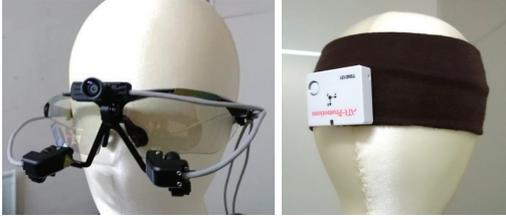
**Fig. 6** Wearable eye tracker and 9D gyro sensor for the experiment. Subjects stare at the stimulus images with wearing the devices.
