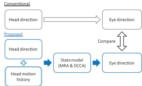
**Fig. 4** Improving the accuracy of eye tracking by head motion history
