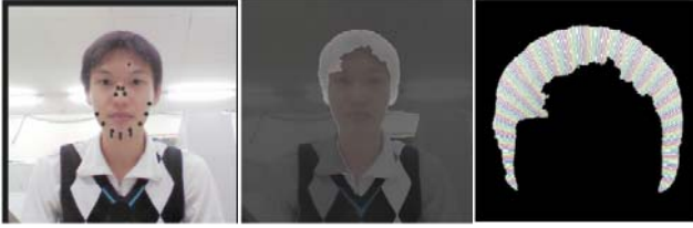
(a) Seeds setting (b) Segmentation results (c) Hairstyle feature vector Figure 4. example of obtaining a hair region and its feature vector
